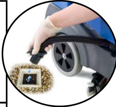
After use, empty waste-water tank using emptying hose and flush-out with clean water. **(A)**
