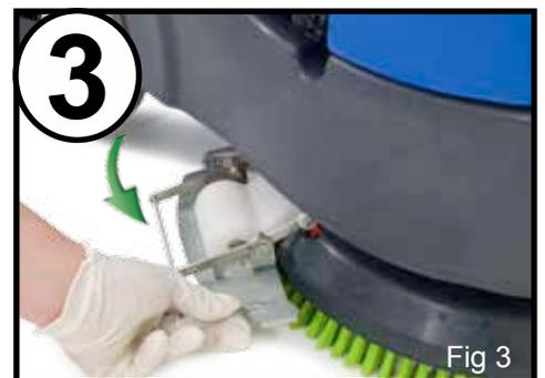
Swing the floor-tool carrier from behind the brush. (Fig 3).
