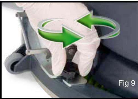
Secure to the carrier using the two knobs fitted to the floor-tool carrier (Fig 9) - (Fig 9a).
