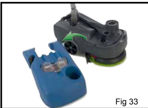
Once emptied the top waste-water tank can simply be lifted off. (Fig 33).
