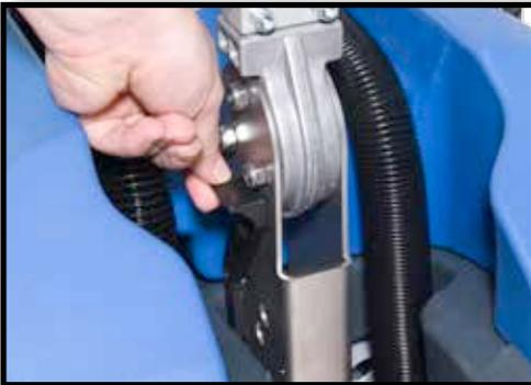
The floor tool carrier can be raised and locked from moving by operating the locking lever, upwards and backwards. this lever can be found next to the lower section of the handle. Unlock and swing the floor-tool carrier to the side of the machine (Fig 8).
