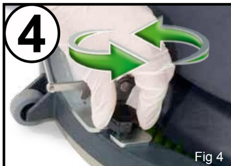
Use the two locking knobs fitted to the floor-tool, secure to the floor-tool to the floor-tool carrier. (Fig 4).
