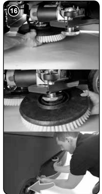
**Featuring the OBS (Octagonal Brush System); the brushes simply push-fit up onto the chucks making fitting and removal a simple process.**
