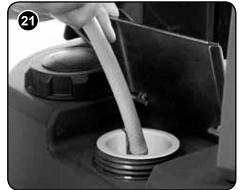
To fill the clean-water tank, lift the cover flap (Fig.19) to expose the filler cap. Unscrew the filler cap (Fig.20) and fill the tank using a hose (Fig.21) or preferred method.
