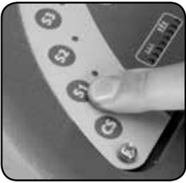
Settings can be stored using one of the three pre-set store buttons (S1 / S2 / S3). Once settings are entered (chemical dose, brush speed and water-flow), press and hold one of the three pre-set store buttons, a light will flash then remain constant; your settings are now saved. This facility can be re-set as often as you wish by simply following the steps above.
