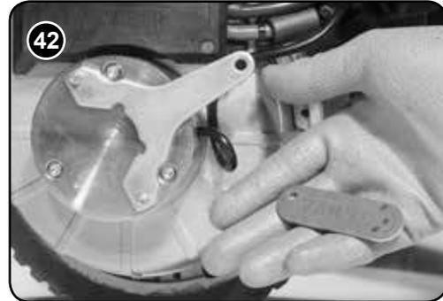
Your start-up kit includes a brake drive disengage key (329945, see Fig.42) which can be inserted between the brake arm and drive housing (see Fig.43).
