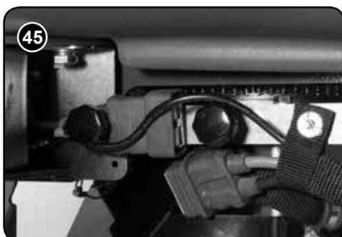
Pull the power connector block apart and refit the two retaining knobs.
