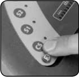
Cleaning Speed setting (CS). When this button is activated the speed is restricted to 3.5 km/h maximum even with the accelerator pedal fully depressed. This is ideal for long cleaning periods. Once this pre-set button is switched-off, the machine will operate at up to a maximum speed of 7.0km/hr.
