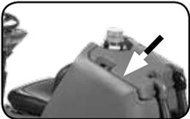
Located in your waste-water (top) tank is a full tank switch, this stops your machine from working once the waste-water reaches its maximum limit. Sometimes the switch gets clogged and blocked, clean to ensure correct operation.
