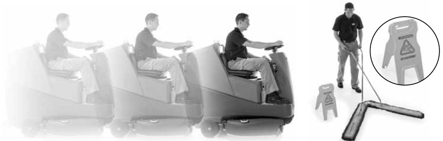
Before performing the cleaning operation, place out appropriate warning signs and sweep or dust-mop the floor.
