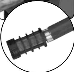
The secondary clean-water tank filter is located to the rear of the battery compartment, and should be checked at regular intervals. Lift white plug and remove the filter, rinse and refit. Ensure tank has been emptied and care is taken when working in the vicinity of batteries.
