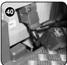
Insert the charging lead required for your country (see start up pack) into the charging point and connect to a suitable power supply (see Fig.40).
