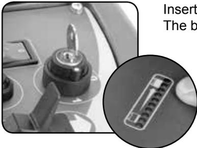
Insert key into main control (on / off) and turn quarter-turn clockwise to position (1) 'ON'. The battery charge level meter will illuminate.
