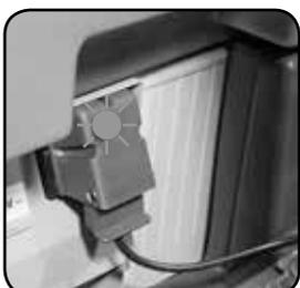
Once mains power is connected the red charging indicator will illuminate. To ensure a full charge, the machine should be left for a period of 12-14hrs. Once fully charged, disconnect the charging lead from both the power supply and the machine.
