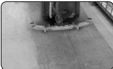
On heavily soiled floors use a 'double scrub' technique. First pre-scrub the floor with the floor-tool in the raised position, allow the chemical time to work then scrub the area a second time with the floor-tool lowered.
