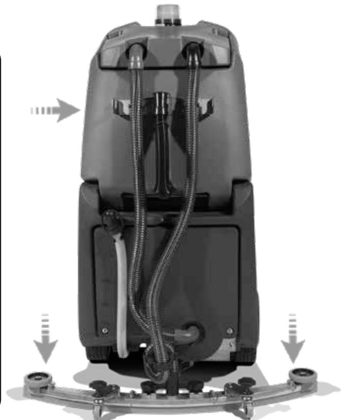
Lower the floor-tool by moving the release lever to the upper position (Fig.29).
