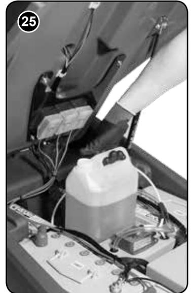
To fill the chemical dosing bottle, first lift up the waste-water tank (Fig.23), remove the dosing bottle, unscrew the bottle cap (Fig.24) and fill with appropriate cleaning chemical. Replace bottle cap, refit dosing bottle (Fig.25) and carefully lower waste-water tank.
