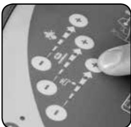
Set Water Flow Rate as required, depending on floor type and level of soiling.
