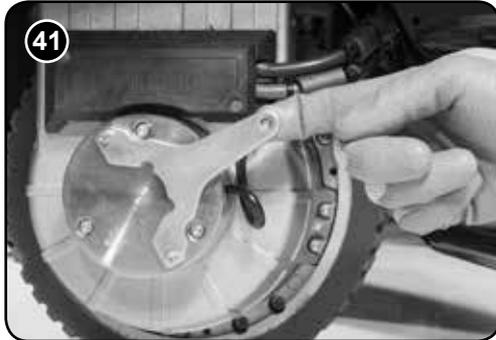
The TTV 678G / 300T is equipped with a free-wheel function that will enable the operator to move / tow the machine. The motor brake is disengaged by opening the brake arm on the side of the drive wheel (see Fig.41).
