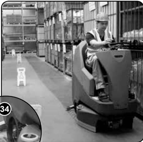
To operate, select forward or reverse, press the accelerator pedal. Vacuum pick-up, water-flow and chemical-dose will turn on automatically and the machine will move forward.
