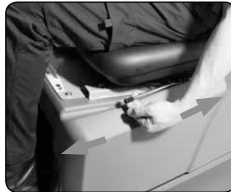
Sitting in the driving position, adjust the seat forwards or backwards as necessary by using the lever found on the left-hand side (see Fig.30).
