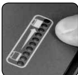
Batteries should be recharged every three months. Charge fully the day before you start using the machine again.
