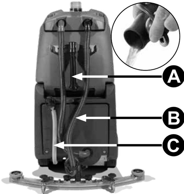
After use, empty waste-water tank using emptying hose **A** and flush-out with clean-water.
