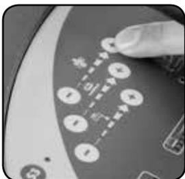
Set automatic Chemical Dosing Mix as required, depending on floor type and level of soiling.
