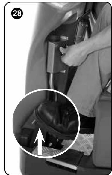
After preparing the floor (see previous section), we are now ready to set the controls to suit the cleaning conditions. Before any settings can be applied, ensure the brush deck is lowered. While depressing left-hand foot pedal (see Fig.26), press down the release lever (see Fig.27) and gently release the foot pedal to lower the brush deck (see Fig.28).
