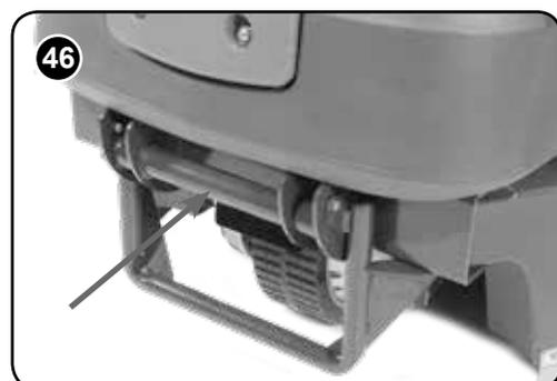
When towing the machine ensure that a suitable tow bar is used.
