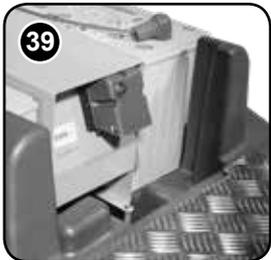
The large capacity gel batteries are sealed for life and are totally maintenance free. The on-board charger automatically monitors the charging process and will switch off when the batteries are fully charged. The machine charging point is located under the top tank. (see Fig.39).
