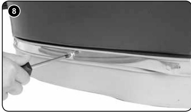
To fit the side pod skirts, first remove the steel retaining strip already fitted to the pod (Fig.7). Align the steel retaining strip within the locating grooves of the rubber skirt and refit using existing screws (Fig.8) Periodically the side skirts should be examined and checked for wear and damage. Replace as shown above.
