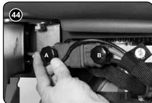
Undo and remove the two retaining knobs (fig.A&B).
