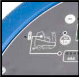
When the waste water-tank becomes full, a red warning light will illuminate on the operator control panel (as illustrated) and the vacuum motor will stop automatically. The waste-water tank requires emptying (see page 17).
