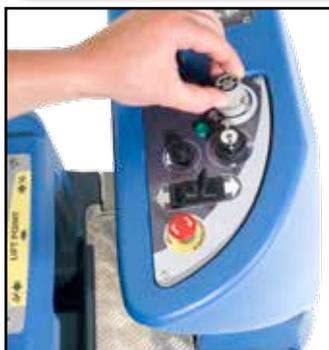
Use the maximum speed control knob and set desired traction speed as required, depending on floor type and level of soiling.
