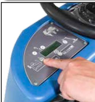
The TTB 3226 has been fitted with a Hi - Lo function, this reduces the noise produced by the vacuum motor by 3dB.
