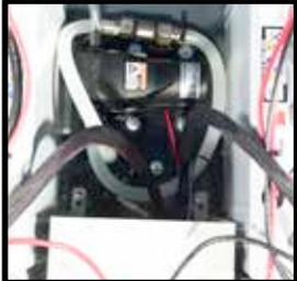
The secondary clean-water tank filter is located to the rear of the battery compartment and should be checked at regular intervals.
