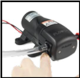
To remove the filter you first have to release the clear tube attached to the pump, move the retaining clip located under the pump and remove the pipe from the pump.
