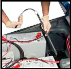
Lift the white plug and remove the filter.
