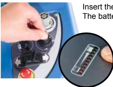
Insert the key into the ignition and quarter-turn it clockwise to the 'ON' position (1). The battery charge-level indicator will illuminate.
