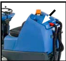
Located in your waste water (top) tank is a full tank switch, this stops your machine from working once the waste water reaches its maximum limit. Sometimes the switch gets clogged and blocked, clean to ensure correct operation.
