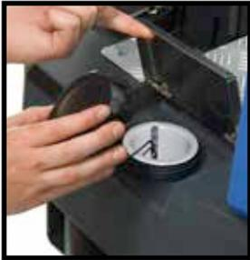
The primary clean-water tank filter is located under the filter cap and should be checked at regular intervals.
