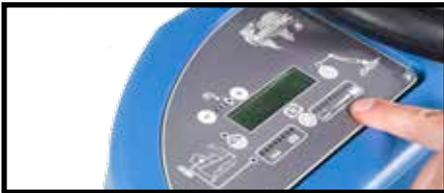
Once the circuit isolator plug has been removed the display panel will show 'INHIBITED' and the machine will not operate.
