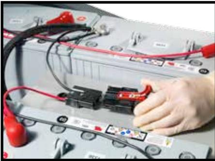
Located under the seat is the circuit isolator plug.
