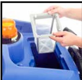
Remove debris basket filter and rinse using clean water, and refit.
