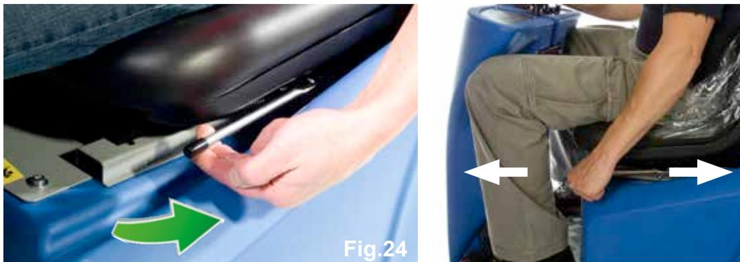
Sitting in the driving position, adjust the seat forwards or backwards as necessary by using the lever found on the left-hand side (see Fig.24).
