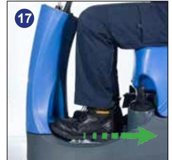
To lower the brush deck slide the brush deck foot pedal forward with your foot (Fig.14) and gently release the foot pedal (Fig.15). The brush deck is now in the lowered position.
