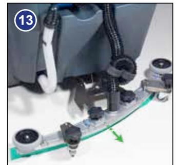
Lower the floor-tool arm by moving the floor-tool lever to the upper position (See above).
