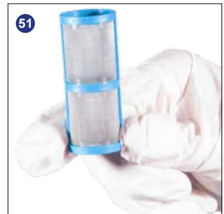
The clean-water tank filter is located to the front of the battery compartment, and should be checked at regular intervals (Fig.49).
