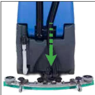
Refit vacuum hose to the Floor-tool when finished.
