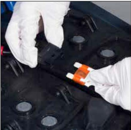
If the machine will be standing unused for a period of 30 days or more, then batteries must be fully charged and battery fuses removed using the Maxi fuse-puller provided, prior to this period.
