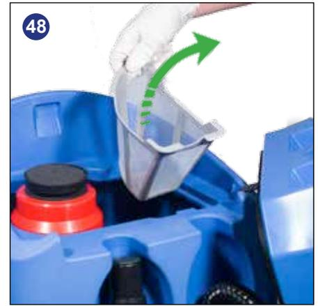
Located in your waste water (top) tank is a vacuum shut off system, this prevents suction when the waste water tank is full. It also prevents foam created by high-foaming detergents from entering the motor. Sometimes the float vents get clogged and blocked, clean to ensure correct operation (Fig.46-47) regularly check and clean the air filter in the top of the assembly.
