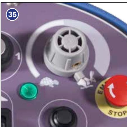
Use the maximum speed control knob and set desired traction speed as required, depending on floor type and level of soiling (Fig.35).
