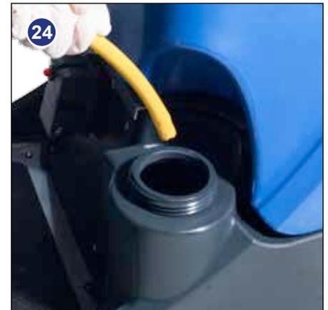
To fill the clean water tank extend the Flexifill hose, remove the rubber seal and fill from a suitable water outlet (Fig.22). Replace seal and hose to original position when finished.
