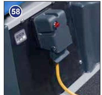
The large capacity gel batteries are sealed for life and are totally maintenance free. The on-board charger automatically monitors the charging process and will switch off when the batteries are fully charged.
