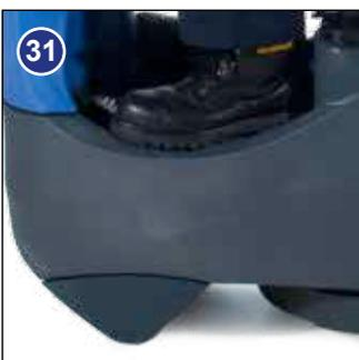
The TTB 2120 is equipped with an Anti-tip system. If the operator attempts to turn a corner when the machine is going at speed, the machine will automatically slow down preventing the machine from tipping over. Additionally the buffers at the front of the machine are designed to prevent the machine tipping in the event of the operator turning sharply (Fig.31).
