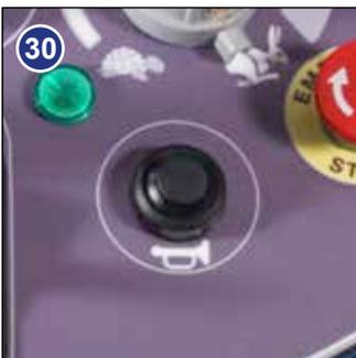
The horn is located on the right-hand side of the operator control panel (Fig.30).
