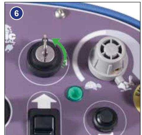
Insert key into ignition and turn quarter-turn clockwise to the 'ON' (1) position, make sure that the forward / reverse switch is set to forward and the speed control is set to low (Fig.4).
