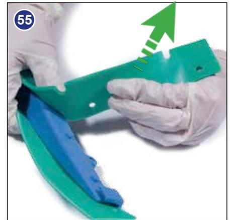
Periodically the floor-tool blades should be examined and checked for wear and damage.
