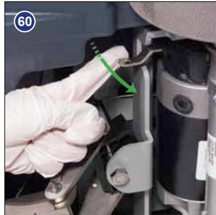
The Free-wheel lever can be found on the right hand side of the rear axle (Fig.59). To disengage the brake, pull the lever into the down position (Fig.60). Re-engage the brake by moving the lever into the up position.
