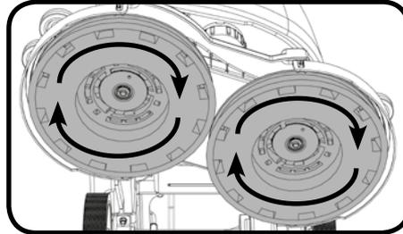
2 x 370mm Brush or a 2 x 360mm Pad on the TGB 8572. Featuring the Nulock brush system. The brush is simply pushed and twisted to lock, making fitting and removal a simple process. Slide the brush / pad under the brush deck. Fit the brush / pad onto the Nulock drive chuck, twist to lock the brush / pad in place.
