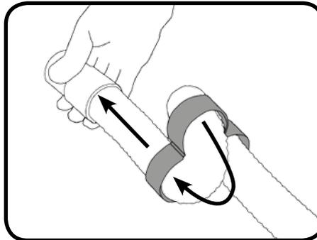
**NOTE: DO NOT** push the vacuum hose onto the floor tool with the floor tool in the raised position.
