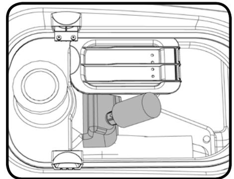
Located in your waste water (top) tank is a full tank switch, this stops the vacuum from working once the waste water reaches its maximum limit. Sometimes the switch gets clogged and blocked, clean to ensure correct operation. Also please ensure float pad is clean and in correct position.
