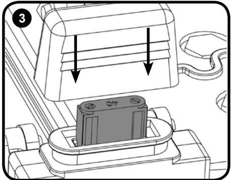
**ENSURE THAT NO METAL OBJECTS COME INTO CONTACT WITH BATTERY TERMINALS WHILE THE BATTERIES ARE EXPOSED. WHEN INSERTING THE FIRST FUSE YOU MAY NOTICE A SPARK, THIS IS NORMAL.**
