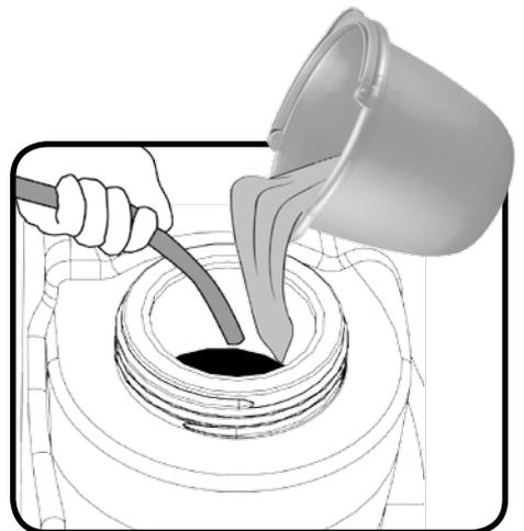
To fill the clean water tank, extend the hose located to the rear of the machine in the centre of the removable filler cap **(1)**. Pull out hose. Open the stopper and place hose under water tap, or use a hose to commence filling. The tank can also be filled by unscrewing the filler cap and using a bucket or similar container **(2)**.
