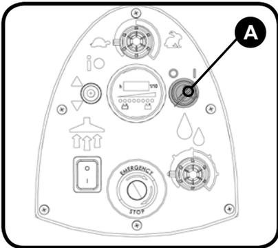
Insert the Ignition key and switch the machine on. **(Fig. A)**
