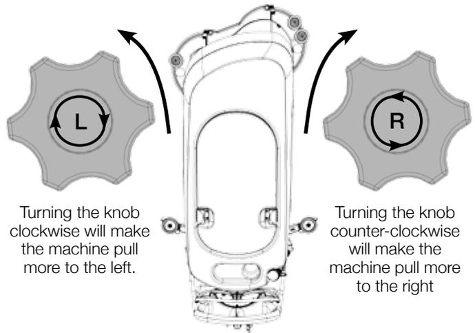
Turning the knob clockwise will make the machine pull more to the left.
