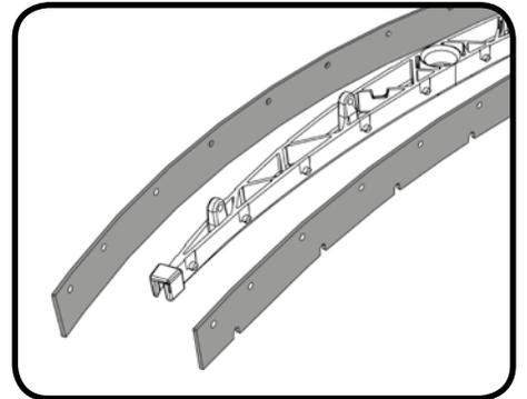
Periodically the floor tool blades should be examined and checked for wear and damage. The blade removal is easy. Simply start by removing the four retaining pins, turn the floor tool over and separate the blade carrier from the body. Peel away the blades from their locating lugs and examine or renew as required. Replacement is a reversal of the removal process.
