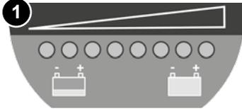
When the machine is getting close to empty the second light from the end starts to flash, the operator should then take the machine to a suitable charging point.
