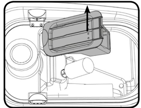
Remove debris basket filter and rinse using clean water, and refit.
