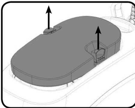
Whilst pressing in the top tank hood toggles, remove the hood. The hood also has a sealing-rubber which should be examined at every clean-down. Rinse using clean water, avoiding the vac filter.
