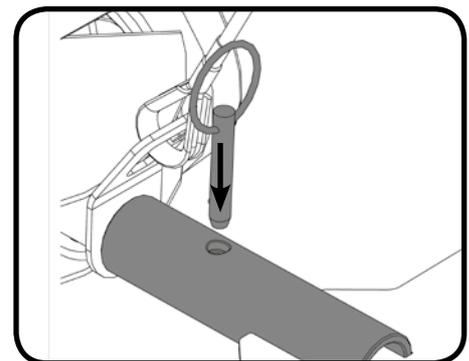
Fit the floor tool and retain using the detent pin.
