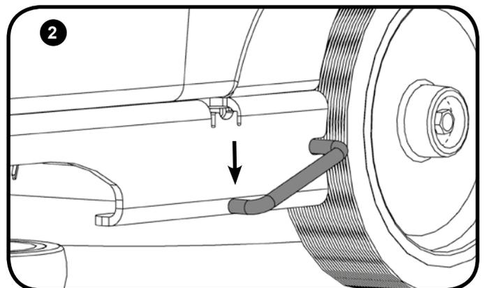
The machine is equipped with a free-wheel function that will enable the operator to move the machine manually if required. The motor brake is located on the right side of the machine near the rear wheel. Pull the arm out (**Fig.1**). Swing to the disengaged position (**Fig.2**). The motor brake will be fully disengaged. The machine will now be in full free wheel mode.
