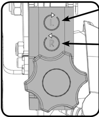
LH Bias: If the machine pulls to the right, turn the knob clockwise to apply left hand bias to the brush deck.
