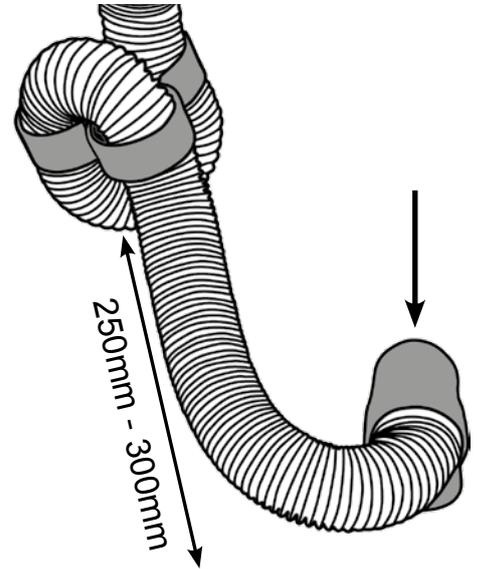
Refit vacuum hose to the Floor tool when finished.
