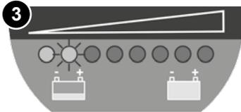
As the machine is used and the batteries are discharged, the meter lights will go out from right to left. If the battery-charge level is allowed to discharge to the point that only the red light remains illuminated, the operator must consider charging the machine.
