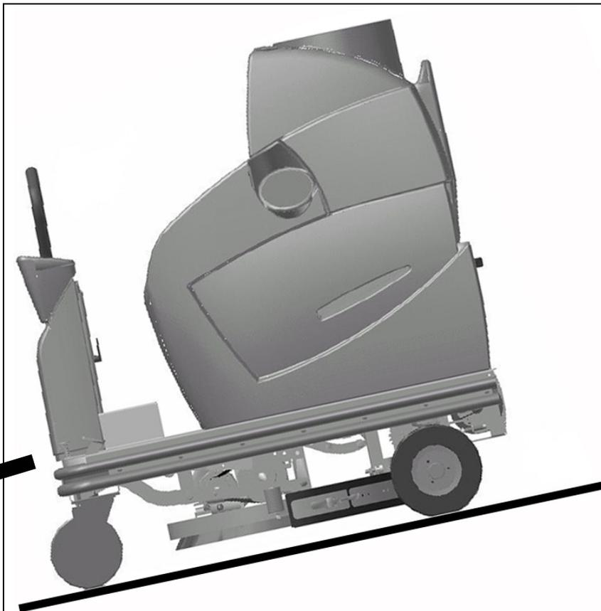
When going down a ramp with the ST360, always go down the ramp forwards.
