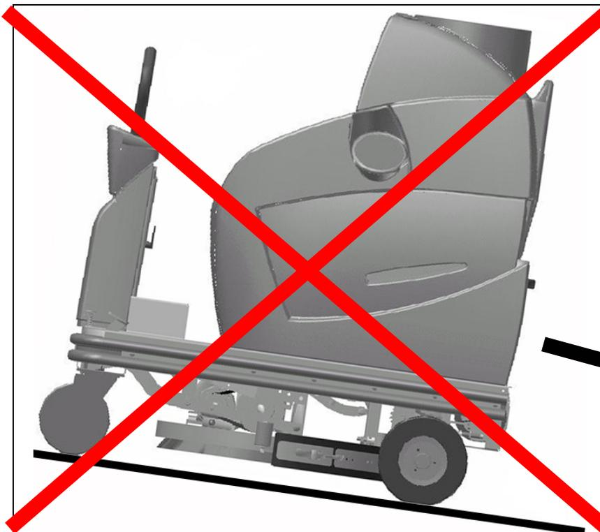
**Note:** If you must unload the machine in reverse, stand in front of the machine and pull the drive levers towards you. Push the machine down the ramp in reverse while continuing to hold the drive levers. **Never** drive the machine down a ramp in reverse. Also, ensure that the battery box is well secured when unloading in reverse.
