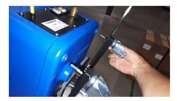
8. Hand thread the bolts back into the machine base, then using the 13 mm socket tighten until snug.
