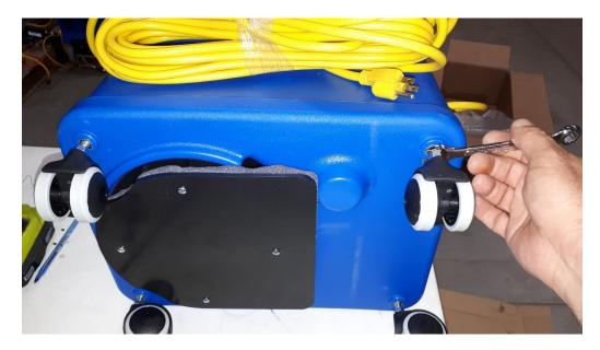
4. Using the cart handle frame and two bases join using the 13mm socket and 13mm wrench
