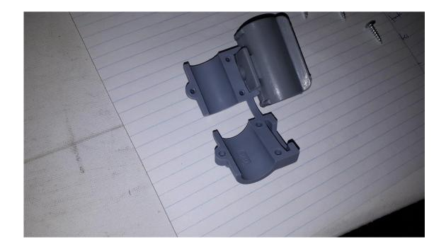
12. Attach grey holder to handle frame using three Phillips screws
