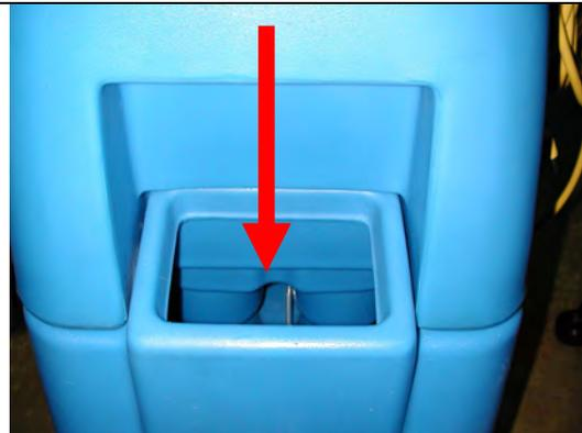
4. Verify that the chemical jug is well connected to the input of the chemical line on the control panel and that it is not empty.
