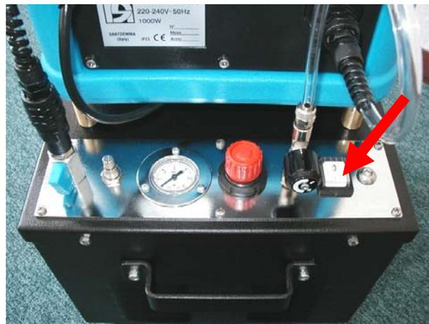
9. Switch on the vacuum motor.
