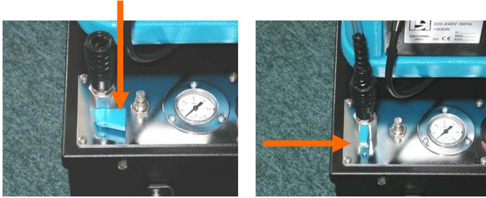
3. Raise the recovery tank, after releasing the spring clips holding it to the solution tank.
