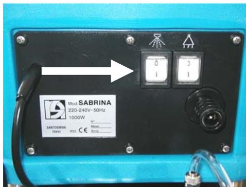
8. Switch the air compressor on by moving the switch to the position “I”. The compressor switch is located on the foam regulation control panel. The compressor will run until full tank pressure is reached (Approx. 1 minute). After this, the compressor motor will only turn on to recharge the tank.
