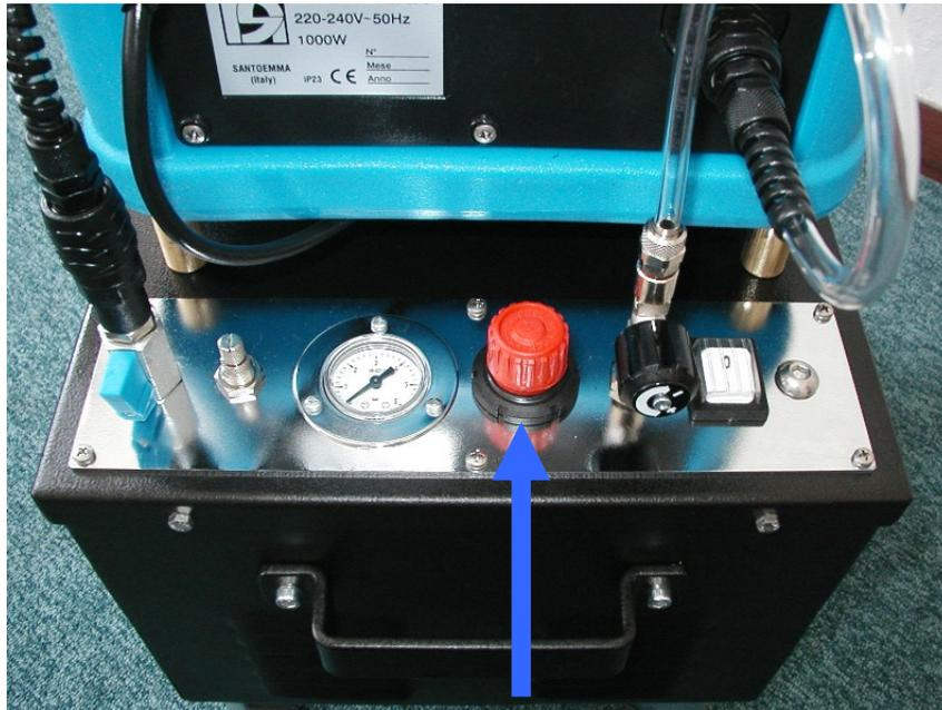
Before making any adjustments, you must wait for the compressor to come up to full pressure.
