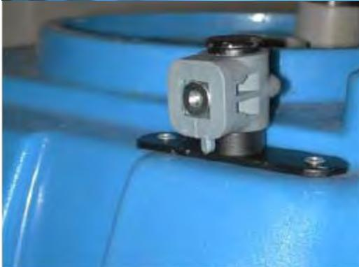
Mounting bracket and Hose holder installed on top left hand side of machine
