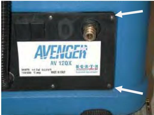
Remove two screws (top right and bottom right) from machine plate as shown.
