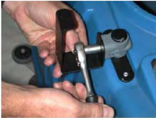
With hose holder and 10mm bolt provided, attach as shown to the left.
