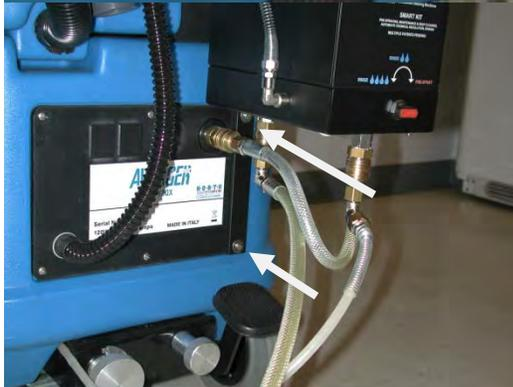
Attach chemical mounting bracket as shown with longer screws and washers provided with kit hardware
