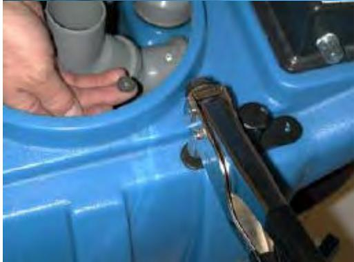
With rivets and washers provided, insert rivet into bracket/tank.
